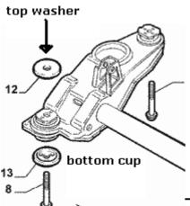
This picture shows the r/h side of the subframe. The top washer is no longer required if you are using the frist line bush 2026
