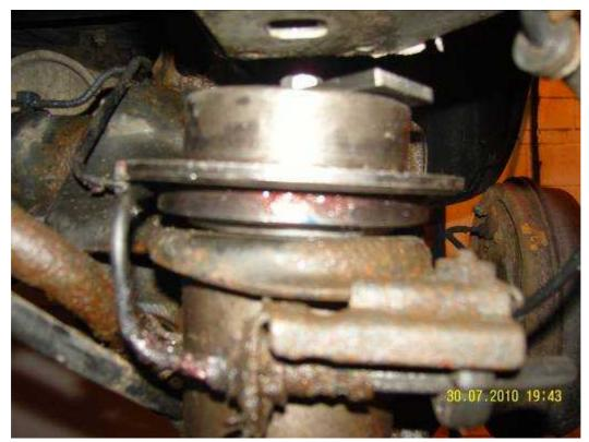
I placed a tool over the bush (a large socket would also do the job) and 'jacked up the sub frame with the tall stand that I had placed under the sub frame earlier. This sandwiched the bush and tool up to the body. I then knocked the sub frame from underneath with a drift to seat the bush, after each strike I took up the weight of the sub frame with the tall stand. After a few blows the bush was seated flush all the way round.
