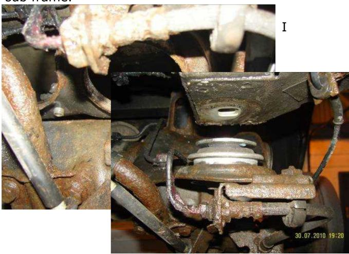
kept checking the fit of the bush in the sub frame to make sure that I did not take off too much metal. When I felt happy that the sizes were good I assembled the bush into a homemade 'press tool' the bush was a tight fit and again it had to come out to open up the hole in the subframe. Second time around it fitted much better. A small dab of loctite was applied to the mating surfaces to help it bond and it was drawn in as far as it would go.
