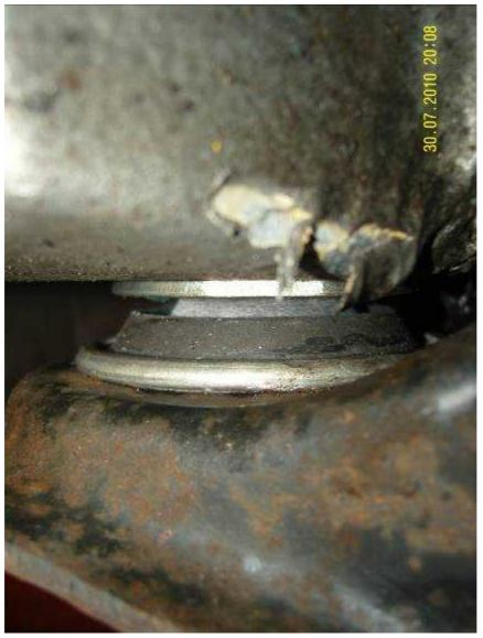
I lowered the stand recovered the tool from the top of the bush and the jacked up the sub frame, copper slipped both sub frame bolts and tightened. I found that the front bolt was now too long as the new bush had the same height from sub frame to body but was a little shorter underneath. As the subframe bolts are metric fine and not that easy to get hold of I packed the bolt with a few washers to take up the extra length. Both bolts tightened, wheels refitted and a
