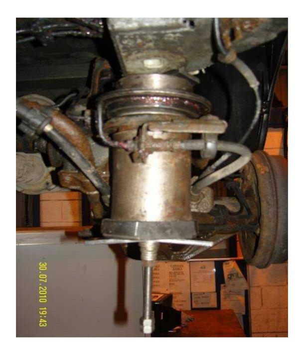
With the tool removed it was apparent that the tool I had made did not get the bush fully into the sub frame. At this point I felt that taking any more from the hole in the sub frame would make the bush too slack in the hole.
