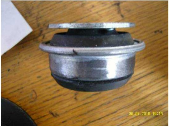
The sub frame hole needs to be 'dressed' with a deburring tool in a drill or a dremel type tool. Basically you need to open the hole in the sub frame by nearly 2mm. what I also did was run the edge of the bush on a bench
