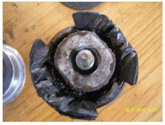
Measurements made with a vernier gauge indicated that the hole in the sub frame measures approx 62mm. The Bravo bush obtained to do the repair measures approx 64mm. Now this bush unlike the old Multipla bush is constructed so that the part of the bush that sits in the sub frame is metal. This means that the bush will be an interference fit which is ideal. But a little on the large side for the hole.
