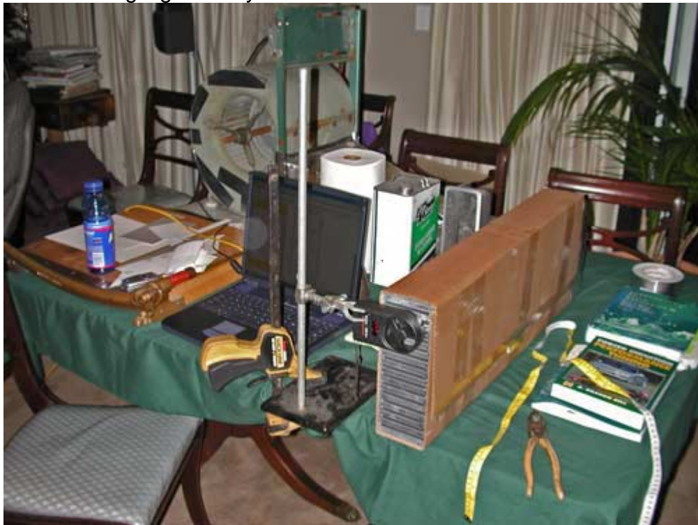
Figure 1.8: Finally a picture of the entire setup, showing wind speed meter mounting.
