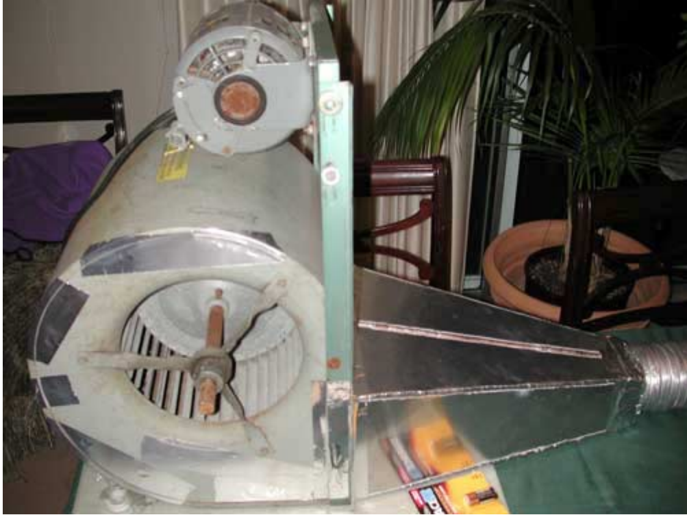
Figure 1.4: Centrifugal blower and fabricated ducting
