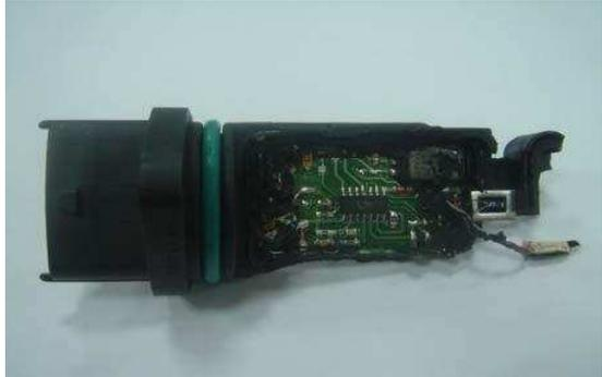
A photograph showing the external view of a counterfeit DMRV. The device is shown from the side, revealing a green PCB with numerous surface-mounted components. The components are mounted manually on a glass-ceramic printed circuit board. |
