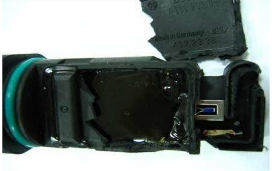
A photograph showing the internal view of a counterfeit DMRV. The black plastic housing is open, revealing a dark, heavily coated PCB. The components are obscured by a thick, black, tar-like substance (bitumen) applied to the board.        |
