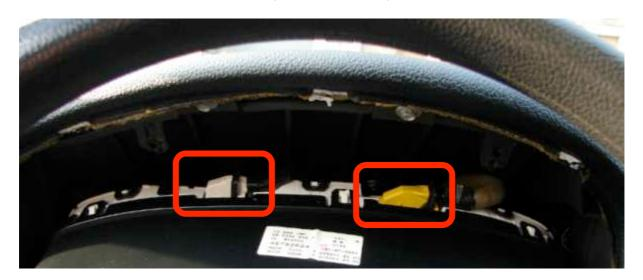
WARNING - AFTER THE CONNECTORS HAVE BEEN REMOVED DO NOT TURN THE IGNITION KEY IN ANY WAY, THE AIR BAG LIGHT WILL LIGHT UP IF YOU DO !!!!!!
