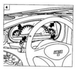
After the abowe is done, remove the dash cover and unscrew these screws.
