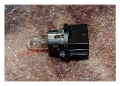
To get the bulb out you need to pull it out of the bulb holder in the arrow direction. Holding the bulb and pulling the bulb holder — or reverse.
